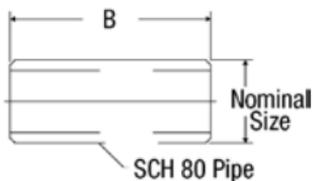
Used for joining any Sch. 80 PVDF fitting face-to-face.
