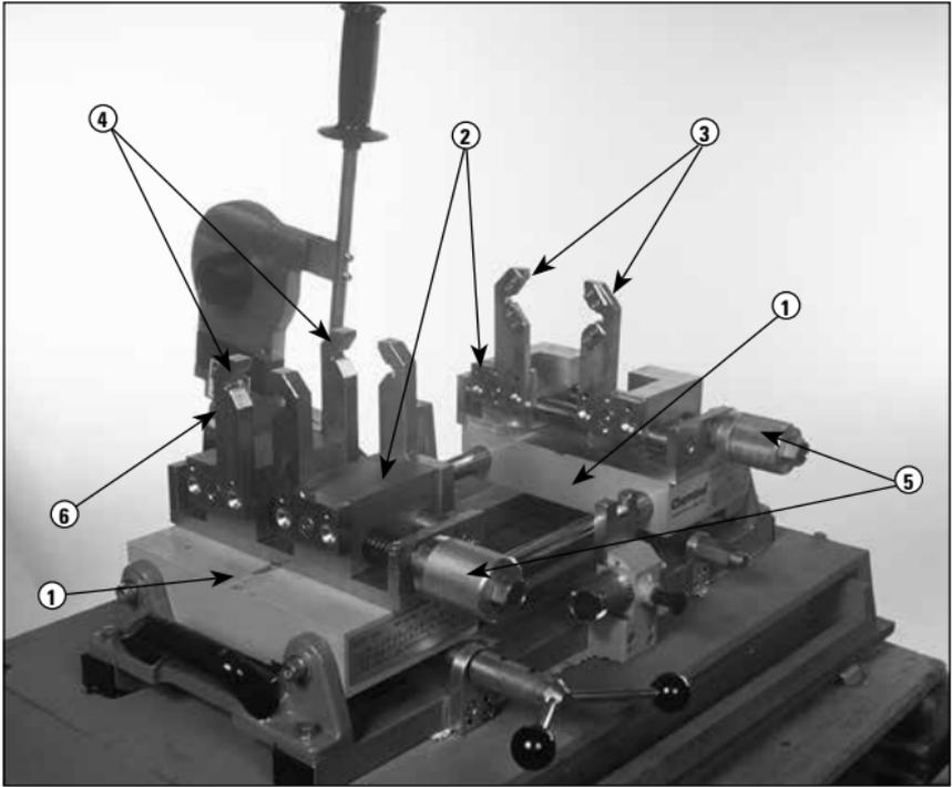
**Features of the Pipe and Fitting Clamping Vises**
