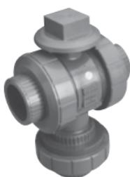
**2" Square Nut Stem Adapter**—Permits operation of a valve with a standard utility (AWWA) wrench. The most common application is for valves located in an underground valve box. The square nut for ball valves is made from PVC. It snaps onto the stem and locks into the slot for turning-stops of a ball valve of any material, in place of its standard handle.
