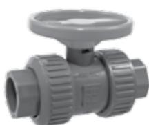
**Round Safety Handle**—Design prevents accidental operation of low-torque ball valve by snagging the lever handle with personal clothing or equipment. Suitable for PVC and CPVC Tru-Bloc® True Union Ball Valves, Model D.
