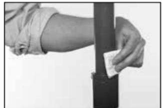
3. Determine the mount of the correct filler rod (see Table, page 36) necessary to make one complete pass around the joint by wrapping the rod around the pipe to be welded. Increase this length enough to allow for handling the rod at the end of pass.
