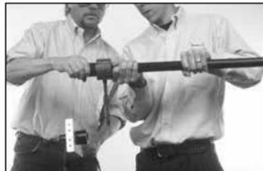
deposits on the Heating Anvils following the making of joints persists, try increasing the silicone spray to thoroughly coat the applicable surfaces and/or reduce the prescribed heating time by increments of 10 – 20%. Be cautious in the reduction of time for sizes 2" and below. Do not waver from the prescribed temperature settings. (See Thermo-Fusion Socket Heating Times.)
