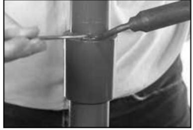
8. Advance the filler rod forward by applying a slight pressure to the rod. Simultaneously applying even heat to the surfaces of both the filler rod and base material by moving the gun with a fanning or arcing motion at a rate of about 2 cycles per second. The hot gas should be played equally on the rod and base material (along the weld line) for a distance of about 1/4" from the weld point.
