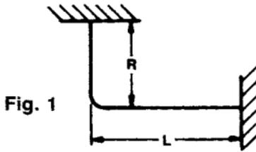
Normally, piping systems are designed with sufficient directional changes, which provide inherent flexibility, to compensate for expansion and contraction. To determine if adequate flexibility exists in leg (R) (see Fig. 1) to accommodate the expected expansion and contraction in the adjacent leg (L) use the following formula:
