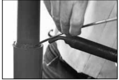
9. Since the starting point for a plastic weld is frequently the weakest part of the weld, always terminate a weld by lapping the bead on top of itself for a distance of 3/8" to 1/2". Never terminate a weld by overlapping the bead side by side.
