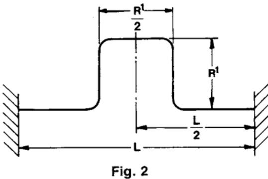
An expansion loop (which is fabricated with 90° elbows and straight pipe as depicted in Fig. 2) is simply a double offset designed into an otherwise straight run of pipe. The length for each of the two loop legs ( $R'$ ), required to accommodate the expected expansion and contraction in the pipe run ( $L$ ), may be determined by modification of the SINGLE OFFSET FORMULA to produce a LOOP FORMULA, as shown below:
